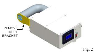
6. Reinstall the bracket screws on the panel box to close the tapped holes. Air hose will be re-attached to the rear frame of the SOUND GUARD SST-E. See Fig. 3.
